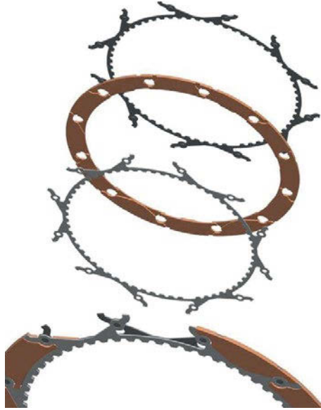
Figure 11 Composite friction Disk construction
