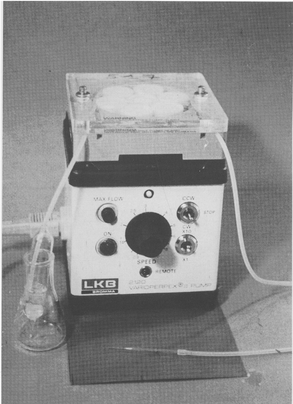
Fig. 5 The system used for transplantation. A micropipette is adapted to a peristaltic pump. The fragment to be grafted can be aspirated into the pipette, placed at its extremity and gently pushed into the host brain.
