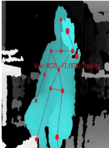
Fig. 2. RGBD camera depth map. Clear pixels are closer to the camera than dark ones. Post processing on this depth map let us extract the viewer silhouette (in cyan) and the viewer skeleton (red dots linked by red lines).
