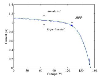
Fig. 3. I-V curves simulated and the experimental
