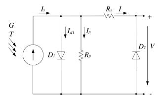
Fig. 1. Equivalent circuit of the solar module
