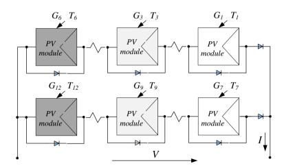
Fig. 4. Configuration for the simulation with partial shading
