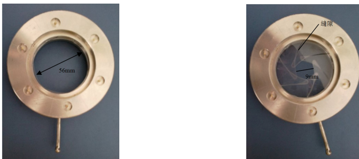
Fig. 6. Adjustable range of fertilizer amount adjusting mechanism in experiment
