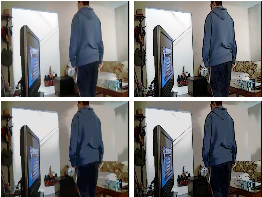
Fig. 5. Frames from the home sequence. Top : Diffusion effect, and diffusion effect with a hand-drawing style. Bottom : Diffusion and quantization effect, and diffusion and quantization effect with hand-drawing style. The radius for the diffusion process is 25 pixels. The quantization parameters are set with a sharpness range between 2.8 and 9.6.
