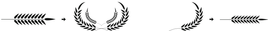
Fig. 1. Left: The skeletal stroke method maps a straight artwork onto a curved path (here: four times). Right: The inverse skeletal stroke method maps a curved artwork into a straight version.
