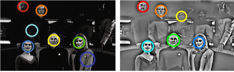
Fig. 1. Detection results using the standard Haar-like detector. Left: Detection results on a “noisy” input image. Right: Detection results on the denoised image.
