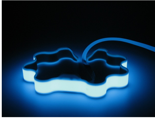
Fig. 2. AM part with integrated EL-Foil and Converter | Fraunhofer IPA
