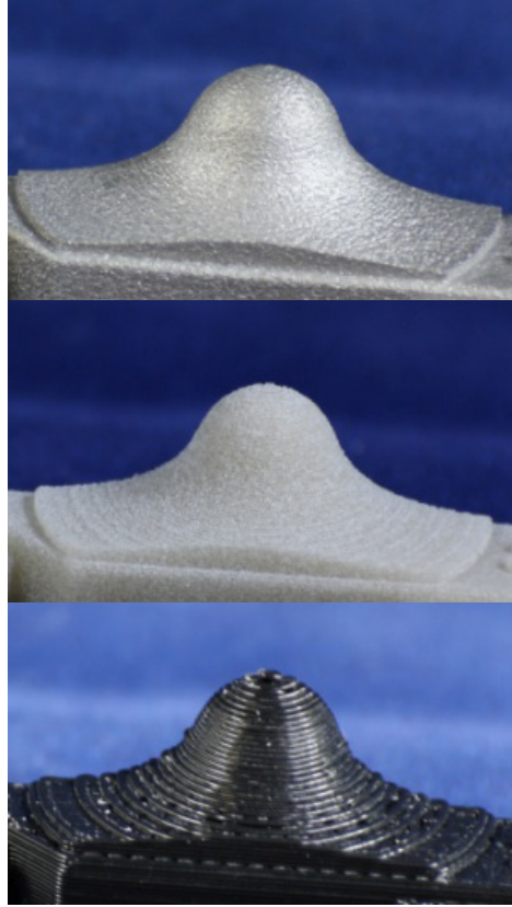
Fig. 18. Comparison of bell-shaped features on the test-specimen built by LBM, LS and FLM
