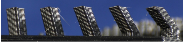
Fig. 16. Angles towards build-platform in FLM
