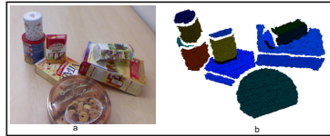
Fig. 1. Primitive Shape Decomposition example : (a) original Point Cloud (b) result of Primitive Shape Decomposition
