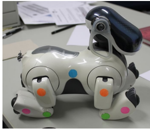
(a) Artificial markers attached to the body surface
