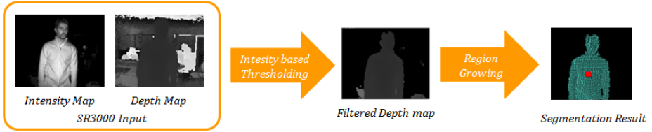
Fig. 1. The main steps of foreground segmentation from the ToF data input to the full body extraction
