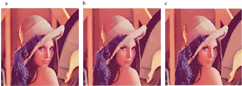
Fig. 4. Another example of color image compression reconstruction. (a) Original image. (b) Region Growing (GL), base color (G) PSNR = 26.0021 [dB], compression ratio 81. (c) Region Growing (RGB), base color (Optimal) PSNR = 26.7238 [dB], compression ratio 83.
