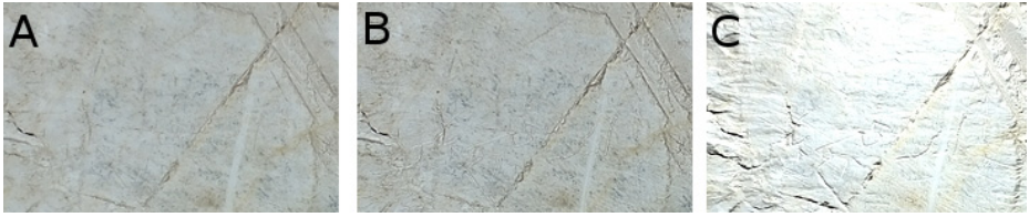
Fig. 5. Detail of the previous image where it is possible to find an inscription. It is not visible using a default light direction (A) and still not visible using filters like unsharp masking on coefficients (B). The static multi-light enhancement makes the lines of interest partially visible.
