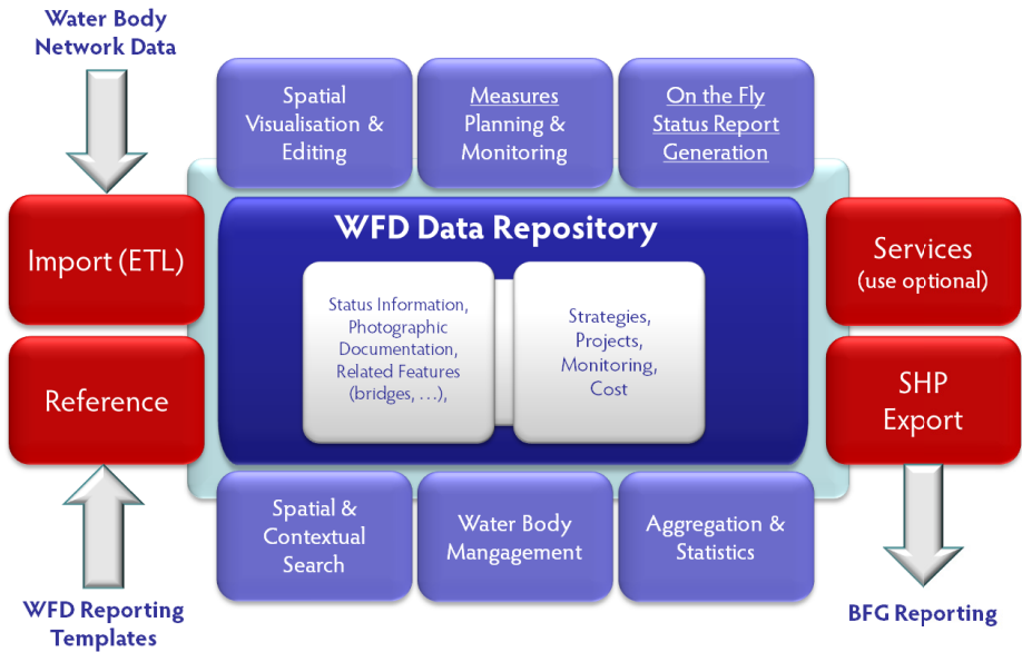
Fig. 3. Overview of functional architecture
