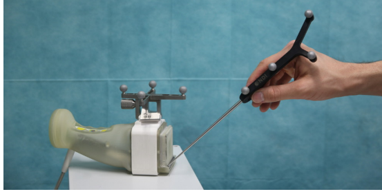
Fig. 3. An optical pointer was used to correlate the detector front face with the optical tracking target attached to the mini gamma camera
