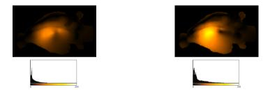
Fig. 5. Surface displacement and histograms with an orange lookup table with the balloon uninflated (left) and inflated (right)
