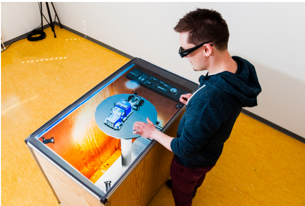
Fig. 7. User interacting with a virtual scene in a stereoscopic multi-touch tabletop setup using touch-enabled 3D widgets. The widgets in the graphical user interface were rendered with negative parallax of up to 10cm height.
