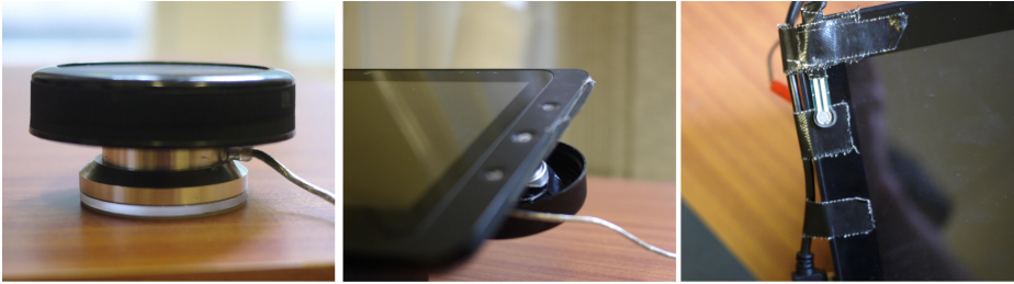
Fig. 2. Hardware setup for our study: Griffin Technologies PowerMate with extended radius (right), the dial affixed to the rear of the tablet (centre) and the pressure sensor affixed to the top-left of the bezel of the tablet (left)
