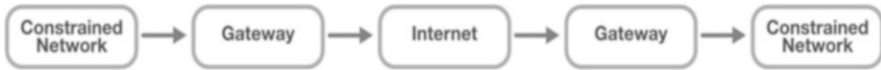
Fig. 7.25 IoT channel for communication over two constrained networks intermediated by the Internet
