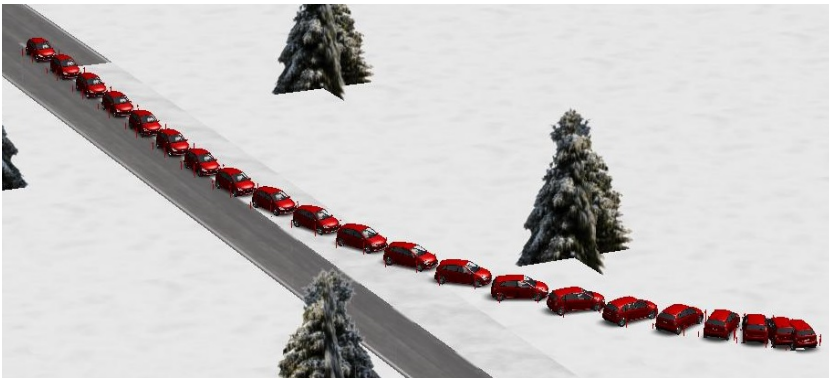
Fig. 8. The consequence of applying the ABS sensor spoofing attack while braking over ice. This simulation shows the position of the attacked car over multiple snapshots of time.
