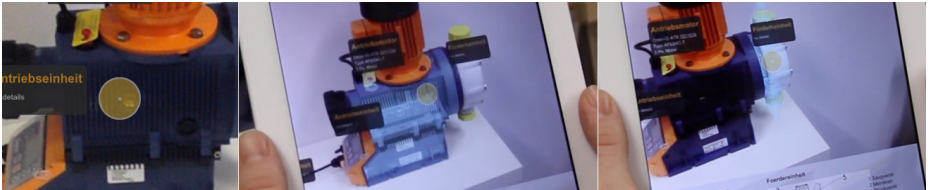
Fig. 1. AR-Gazing: an embodied pointer acts as a visual proxy, where in reality selected components are virtually highlighted
