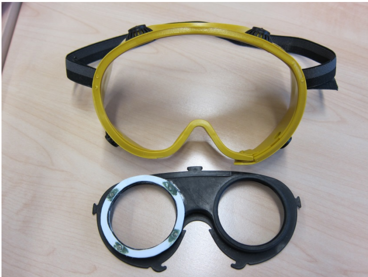
Fig. 1. A standard pair of welding goggles with removable housing and eyepiece was used as the foundation for the chromatic pupillometry goggles (CPG). Each eye socket was outfitted with an polystyrene ring embedded with magnets to allow both the stimulating light sphere and the pupil recording components to click on to the eye in a ‘plug and play’ method.
