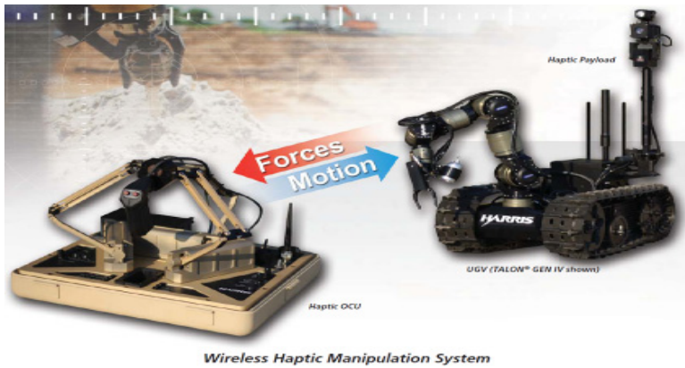
Fig. 4. Harris Corporation's haptic controller
