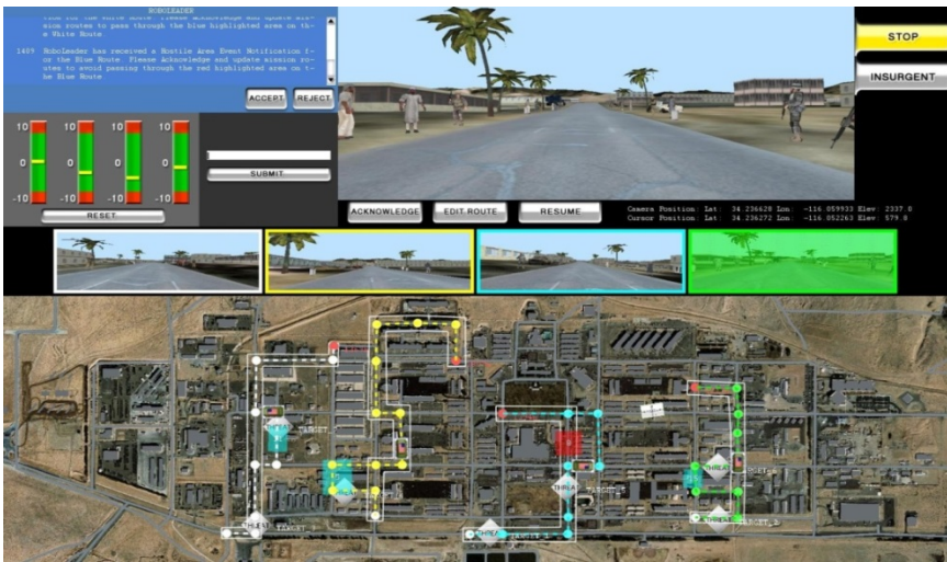
Fig. 2. Simulation scene showing the robot location map, four windows of robot camera views, and a larger display of scene as viewed by robot number 4
