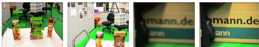
Fig. 2. Example of active STR. From left to right: Localization results after the initialization phase, centering candidate region 1 (a carton box at approximately 3 m w.r.t the camera, the top-left candidate region), after zooming-in, after AAC and auto-focus.
