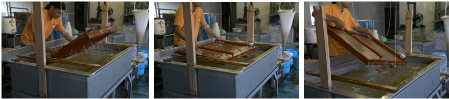
Fig. 1. Three main movements in Japanese papermaking; scooping, swinging and draining (from the left)
