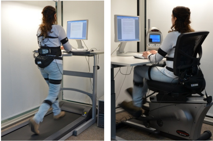
Fig. 1. The Treadmill Desk (left) and the LifeBalance Station (right) in the laboratory set-up with a participant wearing the data capturing equipment
