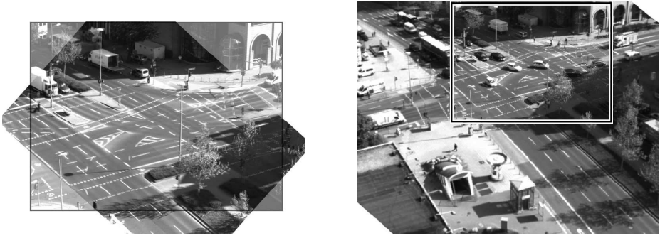
Fig. 7. Registered images: for experiment 1 (left) and 2 (right) based on a homography estimated from learnt point-to-point correspondences
