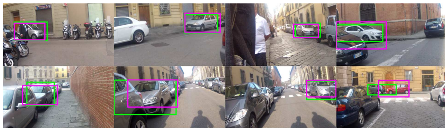
Fig. 1. Mentor-labelled car detections and best overlapping apprentice detections. The green bounding boxes show the labels that the mentor classifier provides for S_e . The purple bounding boxes show the best overlapping detection by the apprentice classifier.
