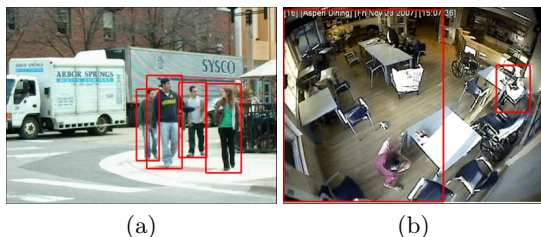
Fig. 5. Typical results of running a state-of-the-art pedestrian detector [12] on the two datasets used in the experiments. On the collective activity dataset (a), the detector performs very well. But on the more challenging nursing home dataset (b), the detector is not reliable since the videos are captured by a fish eye camera, so persons in the videos are not in upright positions. In addition, the video quality is very poor.
