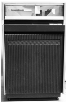
Fig. 9. Disk drive; part of a Control Data model 3200 computer system
