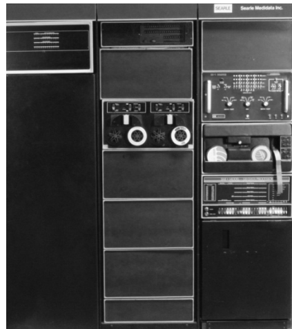
Fig. 14. Searle Medidata Medical Computer based on PDP-8/1
