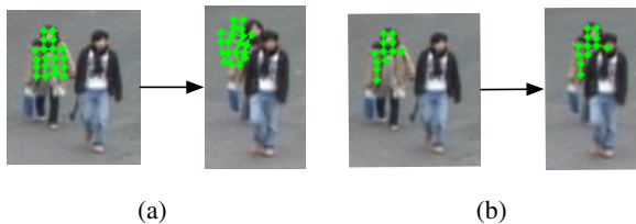
Fig. 1. Tracking examples using two different image block lattices. (a) By using human-like lattice model. (b) By using its pruned lattice model.
