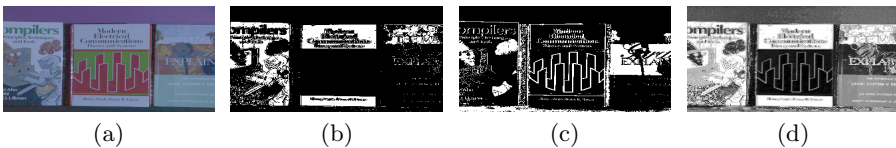
Fig. 1. (a): Image taken under measured illuminant. (b): Light-coloured pixels identified using planar constraint, when correct illuminant is chosen. (c): Putative light-coloured pixels for incorrect illuminant. (d): Analytic Zeta-image (float, 1-intensity).
