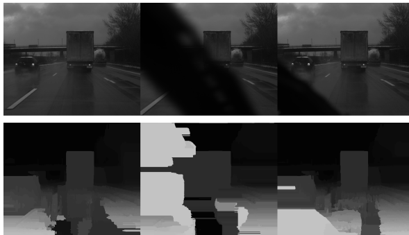
Fig. 3. First row: Three consecutive frames involving large occluded regions and texture inconsistencies, second row: erroneous disparity maps due to imperfections
