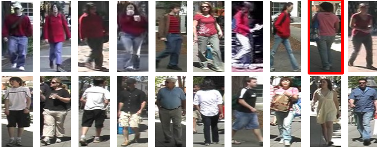
Fig. 4. The top ten images retrieved by MCD 1 , for the “red shirt” (top) and “short sleeves” (bottom) queries, sorted from left to right for decreasing values of the relevance score provided by the detector (classifier). Note that only one non-relevant image is present, highlighted in red.
