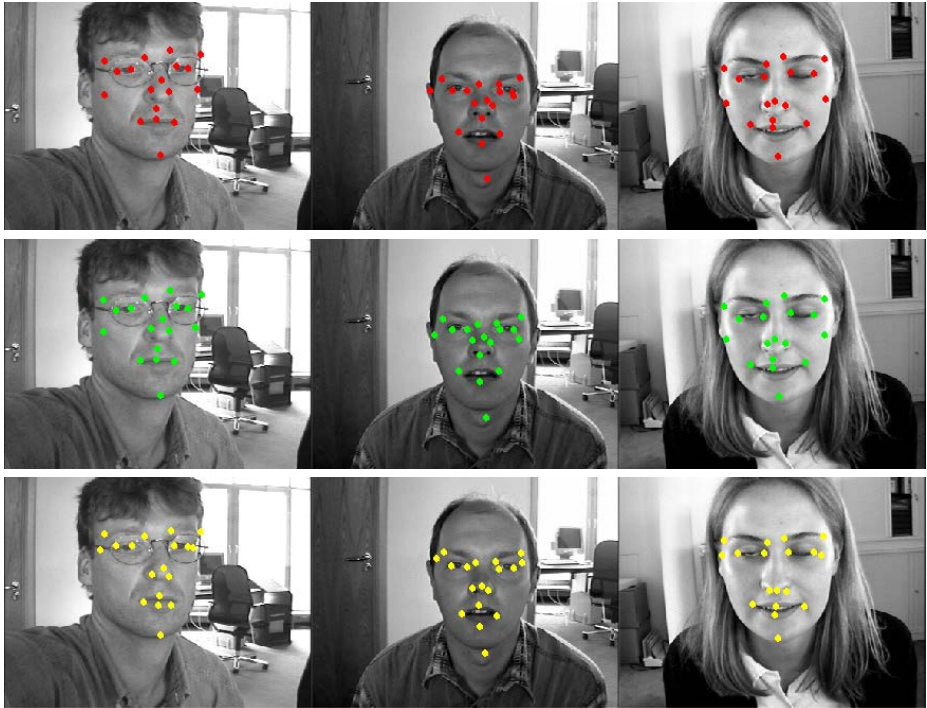
Fig. 5. Images from the BioID database (best viewed in color). First row shows the perturbed landmarks, second row the estimated landmarks using discrete regression (using 100 perturbations), and the third row the estimated landmarks using our continuous regression.
