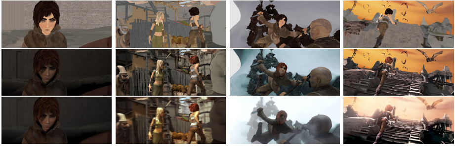
Fig. 2. Render passes. By row from the top: Albedo Pass: Flat, unshaded, surfaces exhibit constant albedo over time. Clean Pass: Illumination including smooth shading and specular reflections adds realism. Final Pass: Full rendering with all effects including blur due to camera depth of field (column 1) and motion (columns 2 and 3), and atmospheric effects (columns 3 and 4). The Final pass resembles the original rendered movie; for a description of changes see [4].
