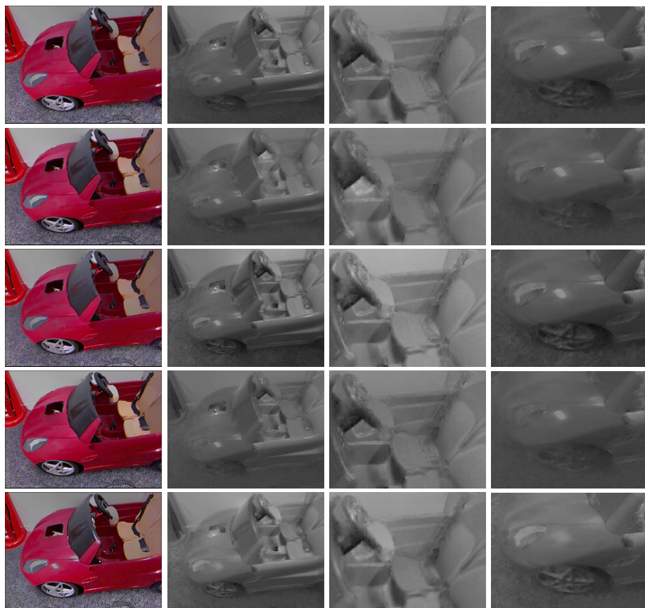
Fig. 6. Decompositions computed using Row 1 the full algorithm; Row 2 without local shading; Row 3 without non-local shading; Row 4 without local temporal; Row 5 without non-local temporal.
