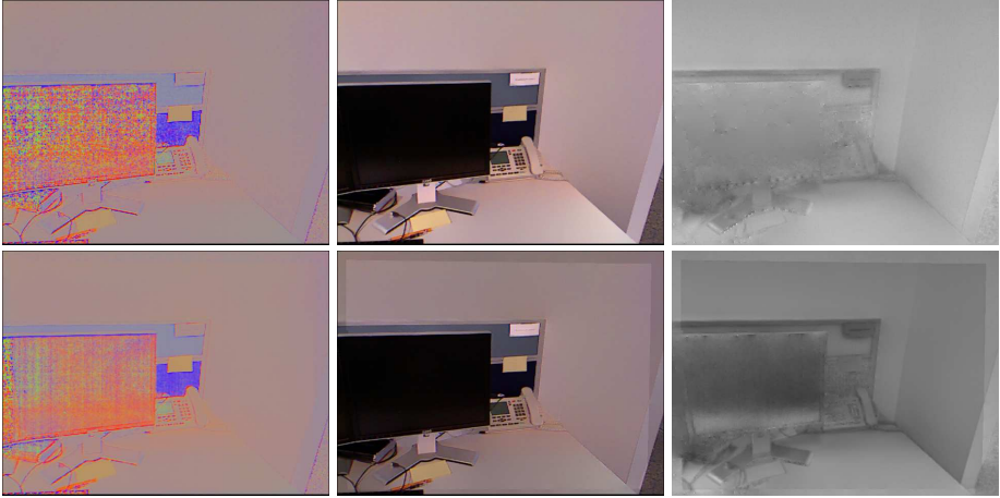
Fig. 4. Result of applying local temporal constraint: Top left original color, shown as chromaticity to better visualize noise effects in dark regions. Top center & right resulting albedo & shading image. Bottom left chromaticity after applying the constraint. Bottom center & right resulting albedo & shading image.
