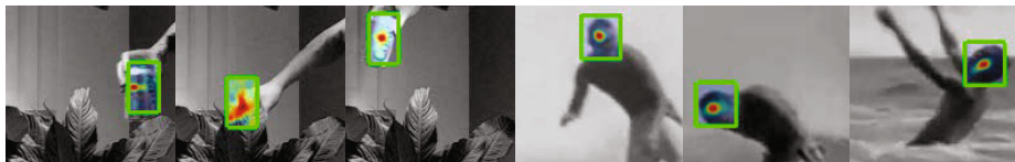
Fig. 1. Example results for coke and surfer sequences, best viewed in color. High values in the response map are red/opaque, low values are blue/transparent. Notice the highly localized responses, except when the target is under occlusion.
