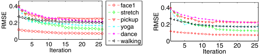
Fig. 2. Reconstruction errors of A2 versus the number of iterations: 2D RIK (left) and aSFM RIK (right). Final reconstructions are obtained with approximately 15 iterations.
