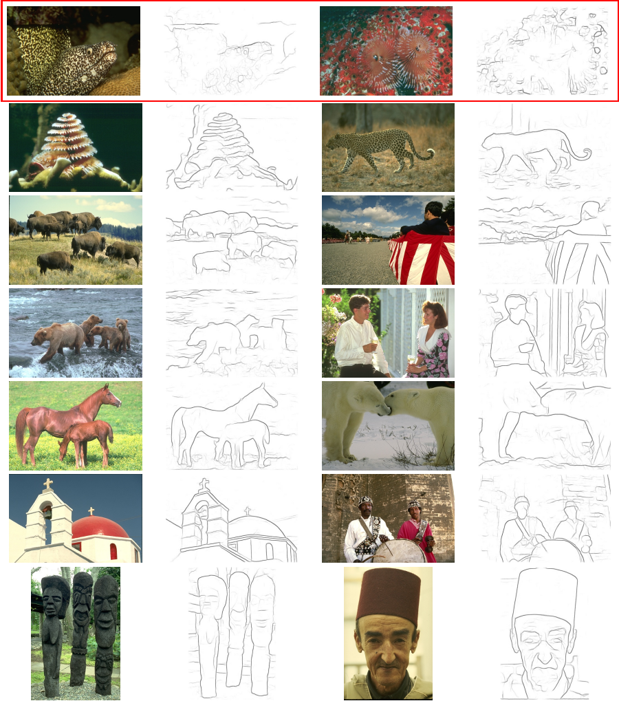
Fig. 4. Examples of contour detections obtained by the proposed PFCF algorithm. Images are from the BSDS300. The top two images outlined in red get two of the worst F-Measure scores.
