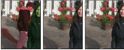
Fig. 4. Weighted average of aligned source frames as guide for the optimization process: (left) target; (middle) average of sources; (right) resulting inpainting composite
