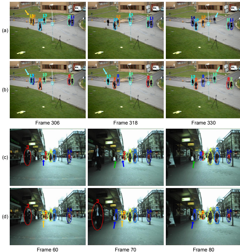
Fig. 6. Comparisons of tracking results with or without category free tracking: (a)(c) show results without CFT, (b)(d) show results on the same sequences with CFT
