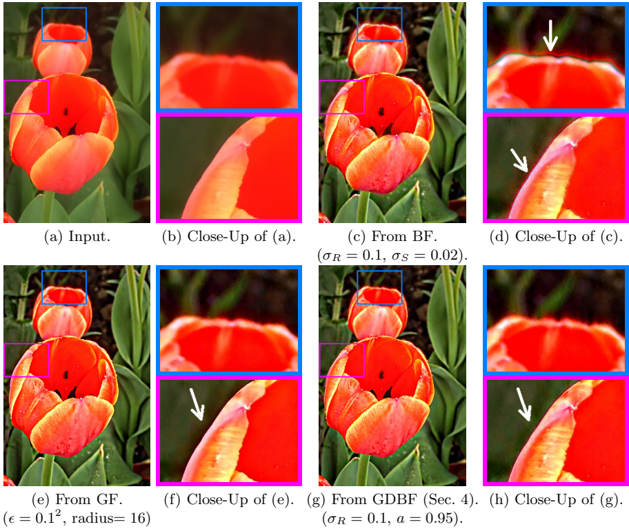
Fig. 4. Detail enhancement. (g)-(h) show that the proposed GDBF removes the gradient reversal artifacts (shown with white arrows) introduced by the bilateral filter in (c)-(d) and the color bleeding artifacts (shown with white arrow) introduced by the guided image filter in (e)-(f).
