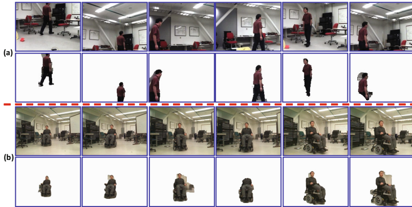
Fig. 6. (a) Detection results on a walking person video for the HM case, (b) Detection results on a moving wheelchair for the FM case. The rows show the original images and MSMS-GBT detection results.
