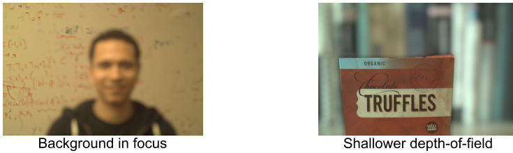
Fig. 7. Synthetic refocusing results. These images were generated by reassigning layers from the depth map to user-specified levels of defocus.
