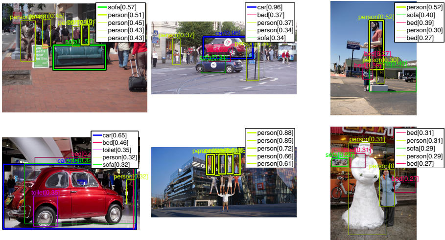
Fig. 5. Qualitative results. The images in the first, second and third columns consist of co-occurrence-violating, relative position-violating, and relative scale-violating images, respectively. In each image, the top-five abnormal objects are represented in bounding boxes.
