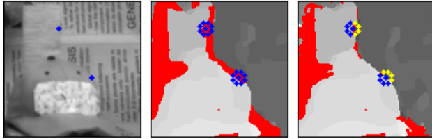
Fig. 3. Application of masks to scenes with occlusions. Left to right: reference image, a depth map after one iteration, and a posterior refinement using masks. Enabled grid points are shown in blue, and disabled grid points are drawn in black. We show a simplified grid of 9 points, for simplicity.
