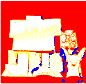
Fig. 8. Benchmarking the spatiotemporal descriptor against occlusions. The image displays the depth error after three iterations with masks, using the Daisy-3D3D approach with 11 frames. The error is expressed in terms of layers: white indicates a correct estimation, light yellow indicates an error of one layer, which is often due to quantization errors, and further deviations are drawn in yellow to red. Red also indicates occlusions. Blue indicates a foreground pixel incorrectly labeled as an occlusion. The plot shows accuracy values at different error thresholds for an increasing number of frames used to compute the spatiotemporal descriptor.
