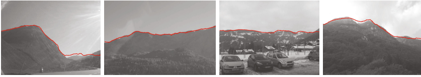
Fig. 7. Some incorrectly localized images. This usually happens to images with a relatively smooth horizon and only few distinctive features. The pipeline finds a contour that fits somewhat well, even if the location is completely off.
